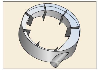
Fig. 5. Tangential vapor horn.
