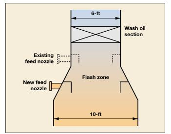
Fig. 6. Recovered lube oil vacuum column flash-zone revamp.
