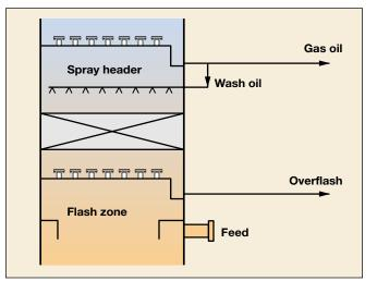
Fig. 1. Typical layout of a heavy oils tower.
