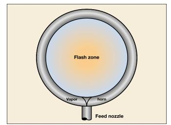
Fig. 4. Radial flow vapor horn schematic.
