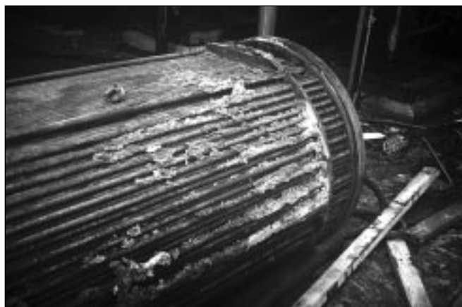
Fig. 6. Fouled overhead exchanger bundle.
