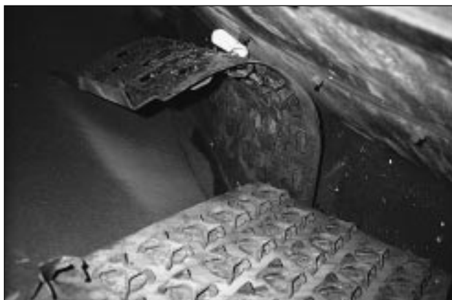
Fig. 4. Stripping and wash section tray damage.
