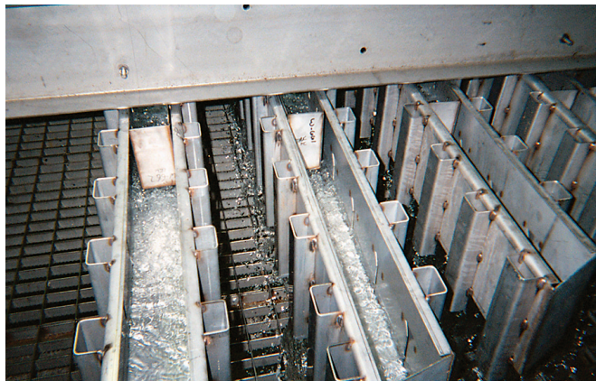
FIG. 9. Revamped main fractionator—view of packing internals.
