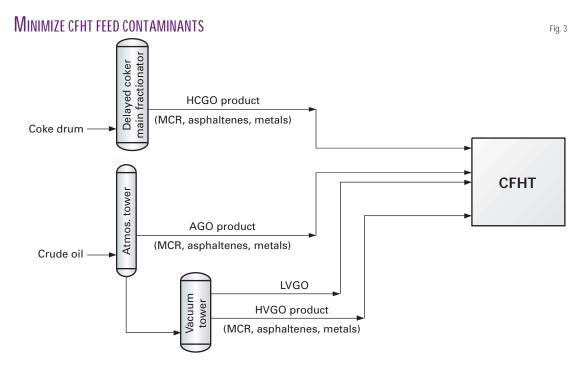
30-ppmw maximum sulfur specification. For example, a decrease in CFHT desulfurization from 98% to 97% can increase FCC feed sulfur from 550 to 780 ppmw. This would raise the FCC gasoline sulfur from 45 to 75 ppm.
