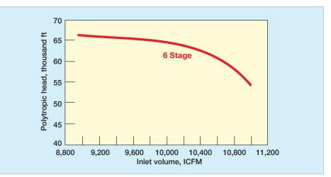
Figure 2 6-Stage Wet Gas Compressor Curve
