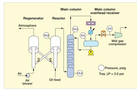
Figure 1 Measured reactor-to-wet gas compressor pressure drop
