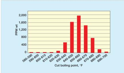
Figure 8 LCO 4,6 DMDBT Distribution by Boiling Range
