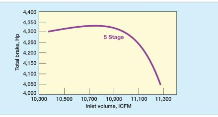
Figure 3 5-Stage Wet Gas Compressor Curve
