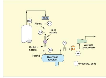
Figure 5 Main Column Overhead System
