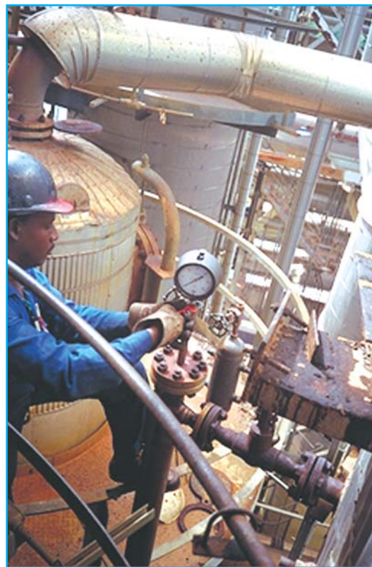
Photo 1. Measure level with pressure
