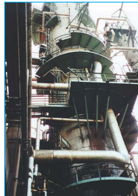
Photo 4. Packed Coker Column
