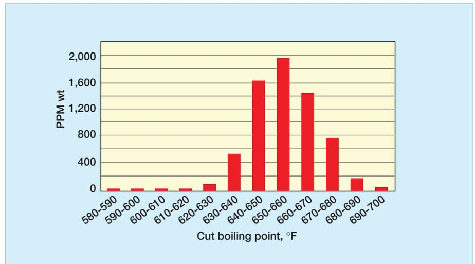
Figure 8 LCO 4,6 DMDBT Distribution by Boiling Range
