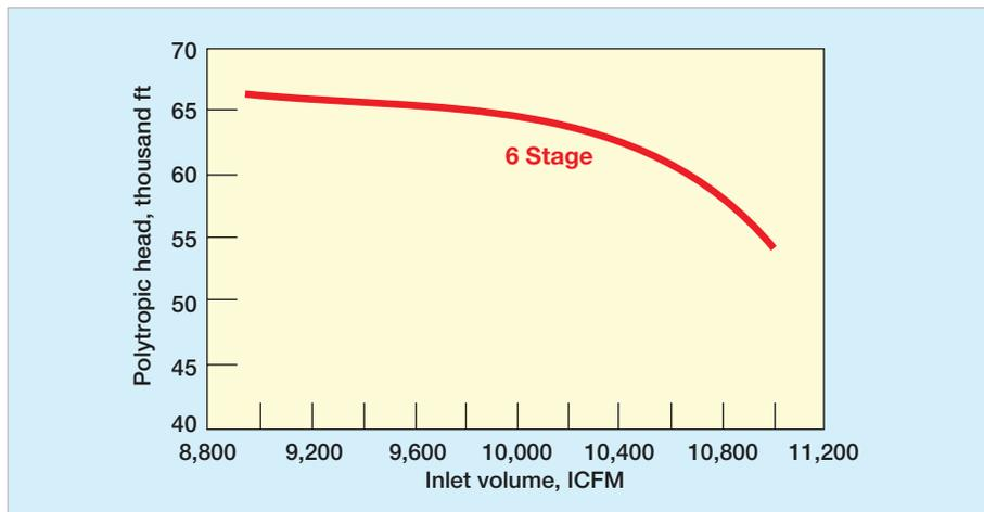
Figure 2 6-Stage Wet Gas Compressor Curve
