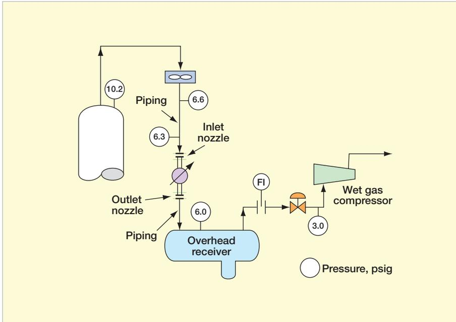
**Figure 5** Main Column Overhead System
