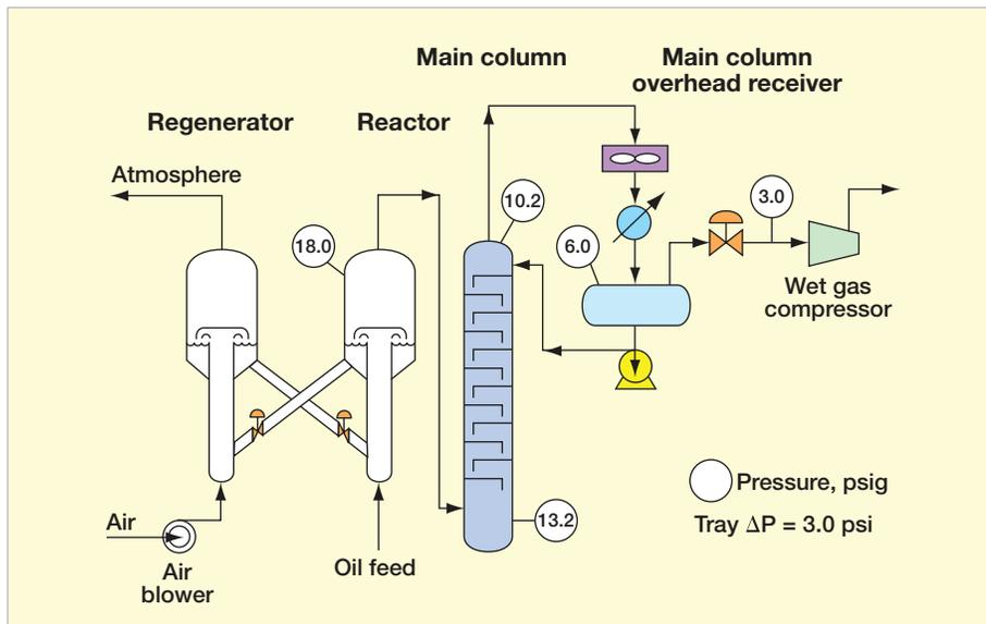
**Figure 1** Measured reactor-to-wet gas compressor pressure drop
