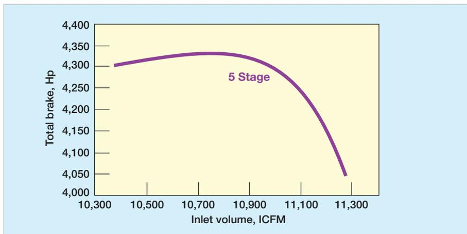
Figure 3 5-Stage Wet Gas Compressor Curve
